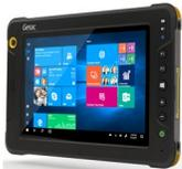
**Certified for Zone 0 Environments:** The EX80 is purpose-built for safe operation in the most hazardous and explosive environments. It is certified for ATEX and IECEx Zone 0 and UL913 (Class I / II Division 1).
