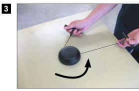
Continue cutting around the antenna to release the entire adhesive pad.
