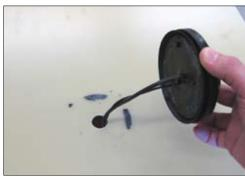
After cutting through the adhesive pad, remove the antenna and disconnect it from the wire harness.
