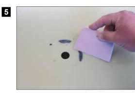
Remove any remaining pieces of the adhesive pad with the plastic scraper.
