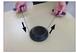
Pull the cable under the antenna and use a sawing action to cut the adhesive pad. (CAUTION! Use care when cutting so you do not cut through the wire harness in the center of the antenna.)
