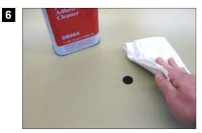
Using a quality adhesive removing solvent and a soft clean cloth to remove any of the remaining adhesive from the vehicle.
