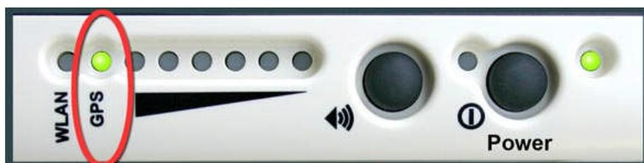
Leave the terminal to acquire a GPS fix. This may take a few minutes. Once the GPS fix has been acquired the GPS LED turns solid green.
