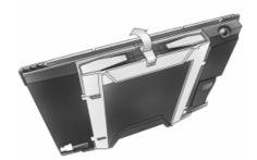
b. Flip up the antenna module and access the keypad and connectors as shown below:
